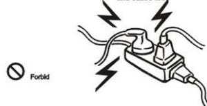
Do not connect a long cable between the plug of power cord and the socket, or the cable may be overheated and cause fire, shock and other accidents.
